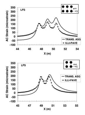
FIG. 12—Comparison of early-life transverse AC strains in LFS section.
