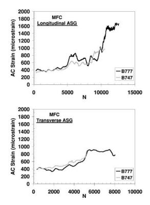
FIG. 5—Peak AC strains in MFC section during trafficking.
