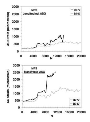
FIG. 6—Peak AC strains in MFS section during trafficking.
