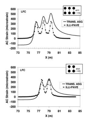
FIG. 11—Comparison of early-life transverse AC strains in LFC section.
