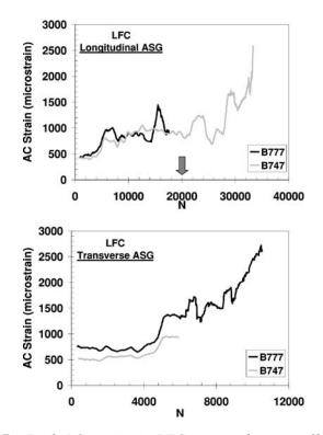
FIG. 7—Peak AC strains in LFC section during trafficking.
