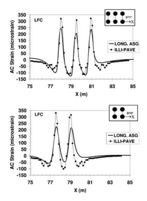
FIG. 9—Comparison of early-life longitudinal AC strains in LFC section.
