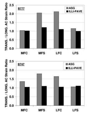
FIG. 13—Comparison of transverse-longitudinal AC strain ratios.
