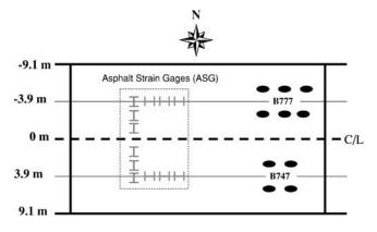
FIG. 3—AC strain gage installation at NAPTF.
