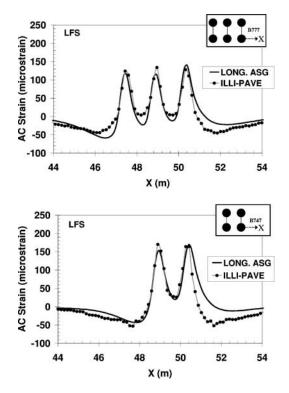
FIG. 10—Comparison of early-life longitudinal AC strains in LFS section.
